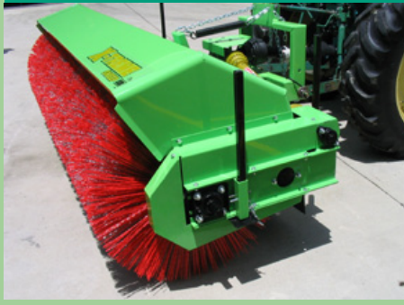
All steel guard protects the drive chain and sprockets
